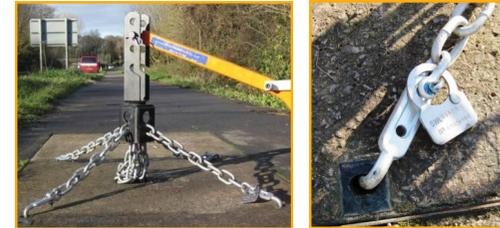
The 10 mm diameter hook on adjustable chain legs allows covers of any shape and form to be lifted.
